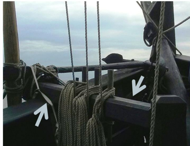
Above Left: Anchor on the bow of Pinta. Above Right: Anchor from the Emanuel Point Shipwreck (Illustration by James W Hunter) Below: The "cathead" (arrows) is a large wooden beam at the bow that supports the anchor.
